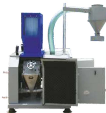
GSC Type 300/300 with integrated blower system
