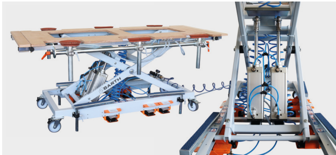
Pneumatically driven lifting table
